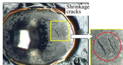
Figure 1 Shrinkage Cracks
