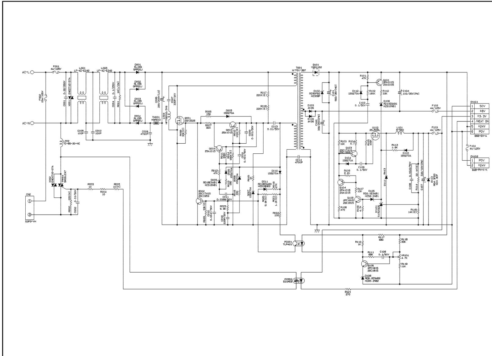
Appendix 4.18 High-voltage Power Supply PCB Circuit Diagram (200V)
