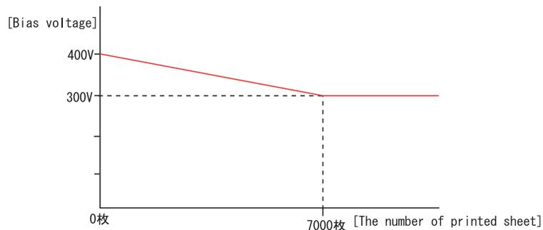
The reason the toner cartridge needs to be replaced from the one (which is empty or near empty) to the new one (which is full of toner) is that the machine is initialized to set developing bias at 400V only when the machine detects the output from both the front cover sensor and the toner sensor when the user replace the toner cartridge.
