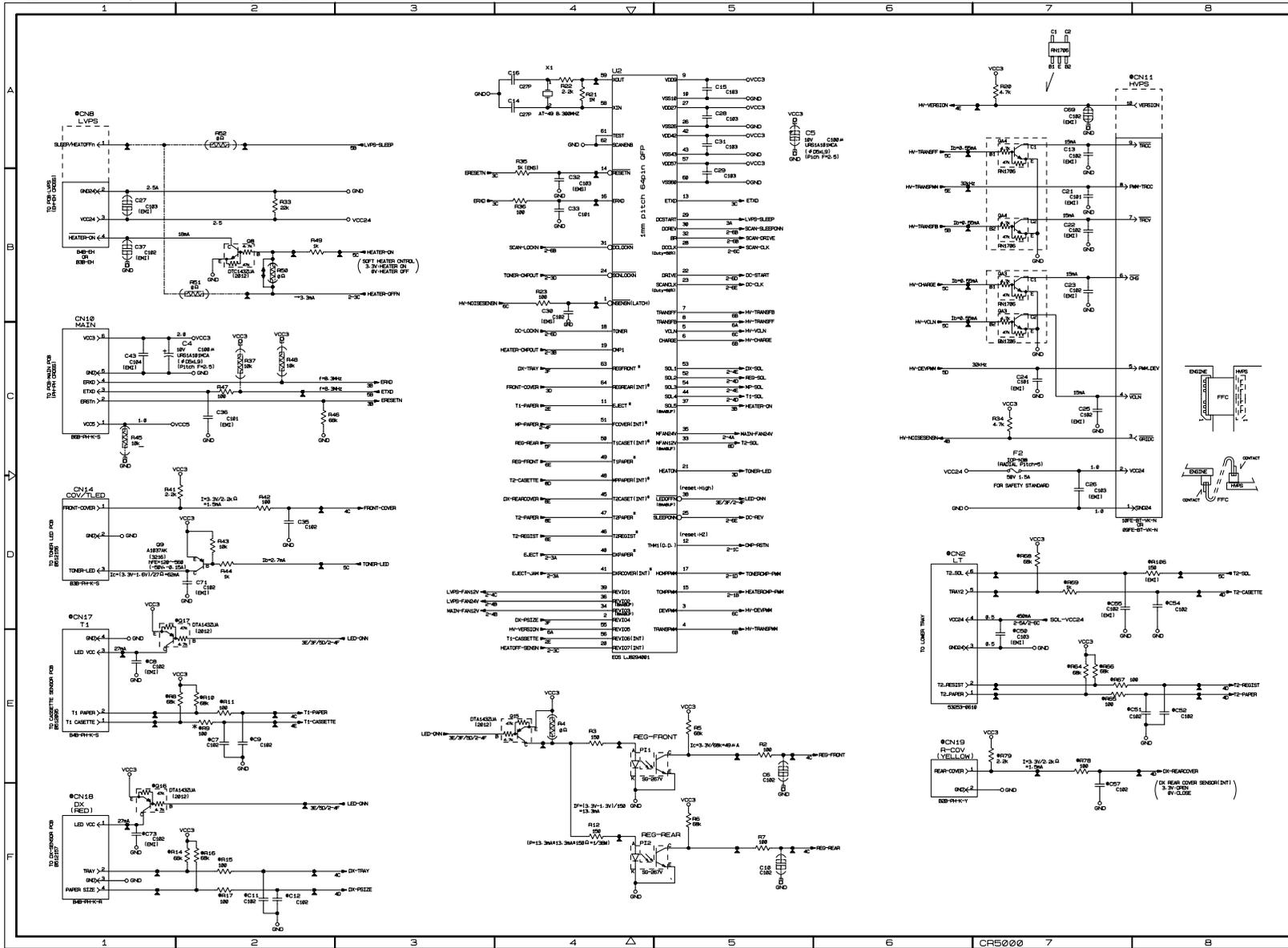
Appendix 4.17 Low-voltage Power Supply PCB Circuit Diagram (100V)
