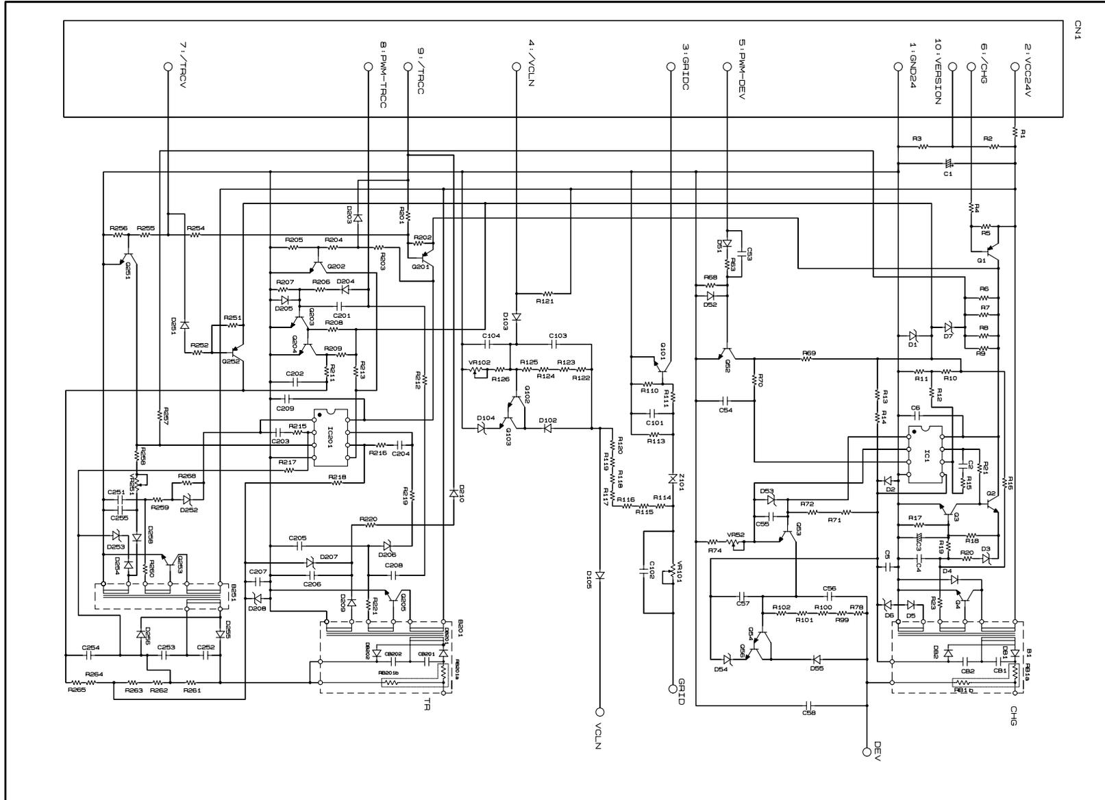
Appendix 4.19 High-voltage Power Supply PCB Circuit Diagram (100V)
