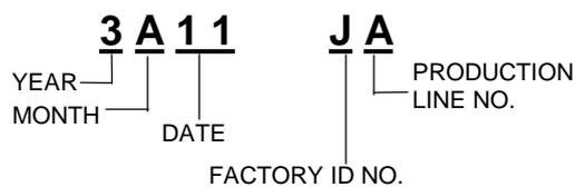
(3) Drum unit: Printed on the bar code label attached inside the drum unit
